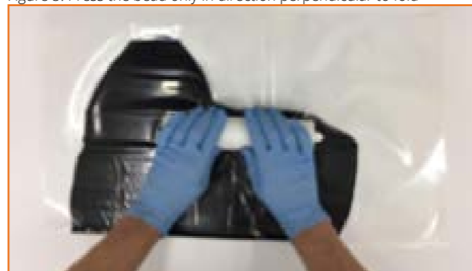
Figure 5: Press the bead only in direction perpendicular to fold
