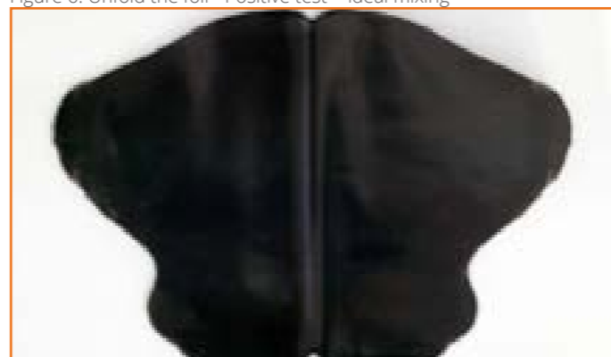
Figure 6: Unfold the foil - Positive test = ideal mixing
